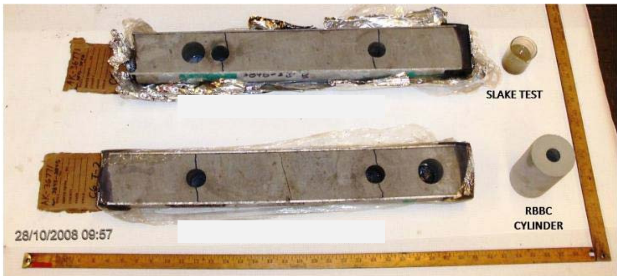
Figure 3-4: Tube samples of Ugnu Clay used for resedimentation (Jones 2010)
